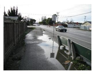
uneven pavement near the bus stops created large splash zones when buses passed by and deep mud divots when buses pulled into a bus stop. Public transit riders had to navigate this ponding water and deep mud simply to board a bus.
