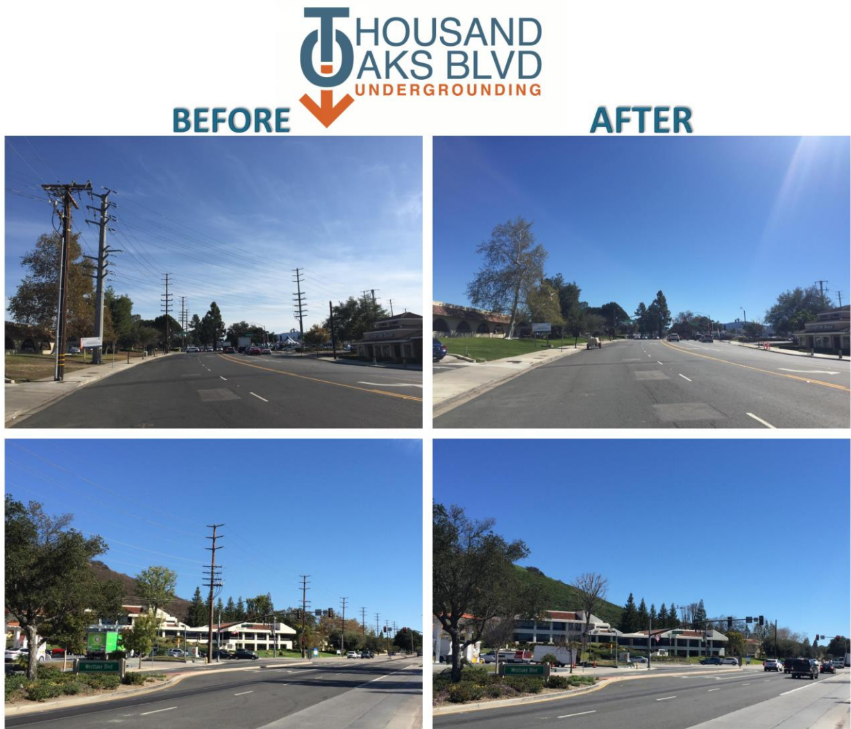
Figure 11 – 2 Separate Views of Thousand Oaks Blvd (before and after the undergrounding project)
