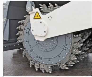
Above: Reclamation Milling drum utilized for mixing and injecting stabilizing agents into existing soils. The Madonna FDR project recycled 18 inches of existing material.
