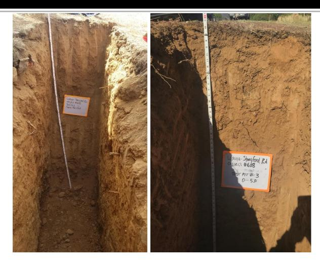
**Project included logging** and sampling six test pits to approximately a 5-foot depth, Dynamic Cone Penetrometer (DCP) testing six locations. Subsequently, geotechnical laboratory testing, engineering analyses, and submission of a geotechnical report with recommendations for pavement repair alternatives were completed.
